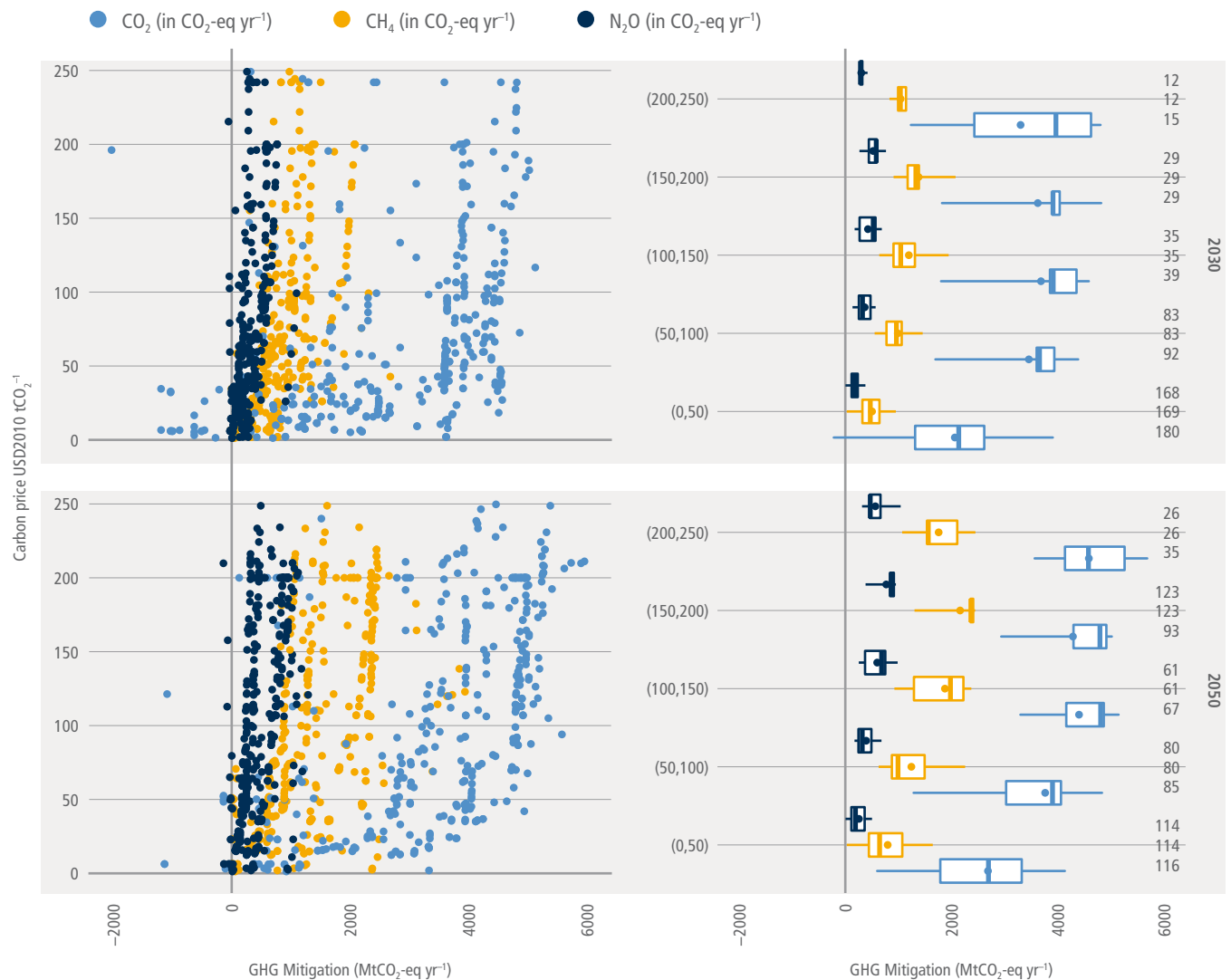
Figure 7.15 | Mitigation of CO 2 , CH 4 and N 2 O emissions (in CO 2 -eq yr -1 using IPCC AR6 GWP100 values) from the AFOLU sector for increasing carbon price levels for 2030 and 2050. In the left-hand panels, single data points are generated by comparing emissions between a policy scenario and a related benchmark scenario, and mapping these differences with the respective carbon price difference. Plots only show the price range of up to 250 USD2010 tCO 2 -eq -1 and the mitigation range between -2000 and 6000 MtCO 2 -eq yr -1 for better visibility. At the right-hand side, based on the same data as left-hand side panels, boxplots show medians (vertical line within the boxes), means (dots), 33%–66% intervals (box) and 10%–90% intervals (horizontal lines). Numbers on the very right indicate the number of observations falling into the respective price range per variable. A wide range of carbon price induced mitigation options (such as technical, structural and behavioural options in the agricultural sector, afforestation, reforestation, natural re-growth or avoided deforestation in the LULUCF sector, excluding carbon capture and sequestration from BECCS) are reflected in different scenarios.
