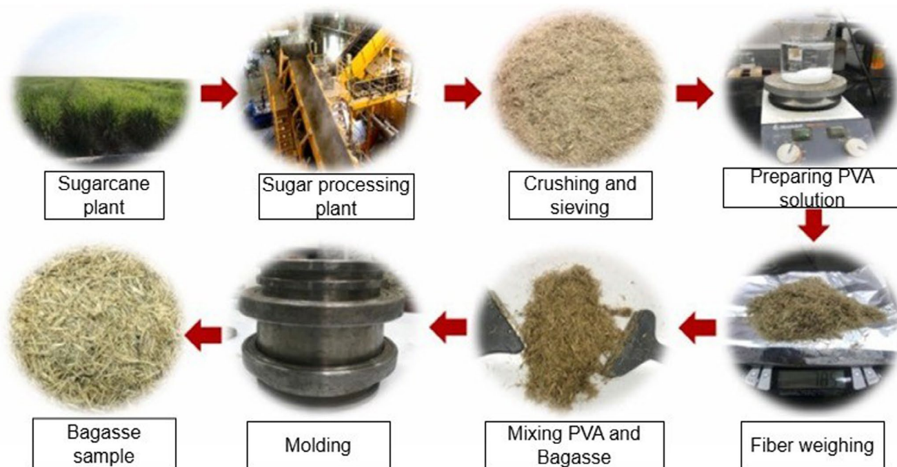
FIGURE 8 | Different preparation stages of sugarcane bagasse waste samples for the development of thermal insulation and sound-absorbing building materials.
