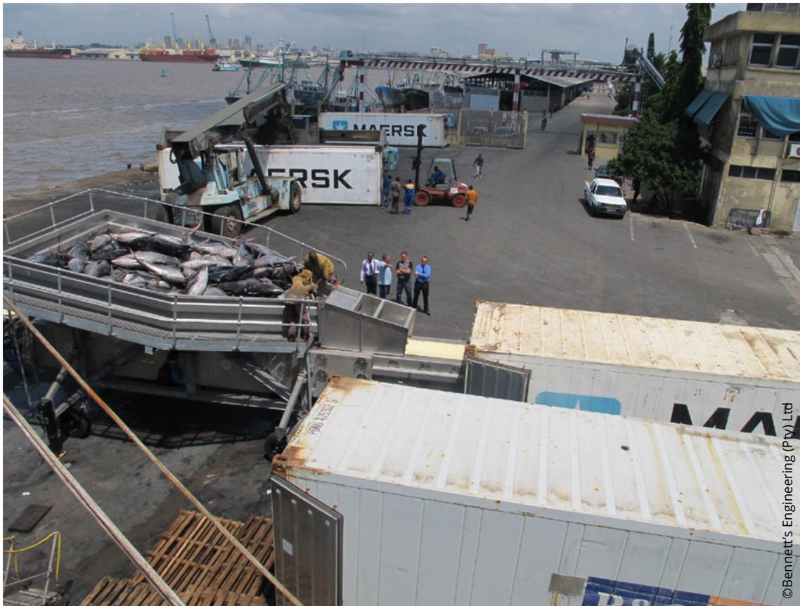
Note: The image shows a retractable conveyor belt and hydraulic operations.
