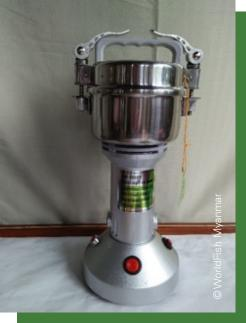
Multifunction grinder used to produce SIS powder
