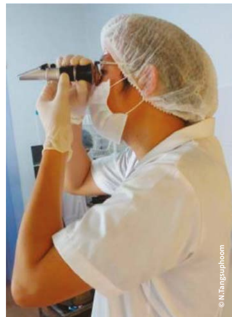
Using a refractometer to measure total soluble solids in the finished product
