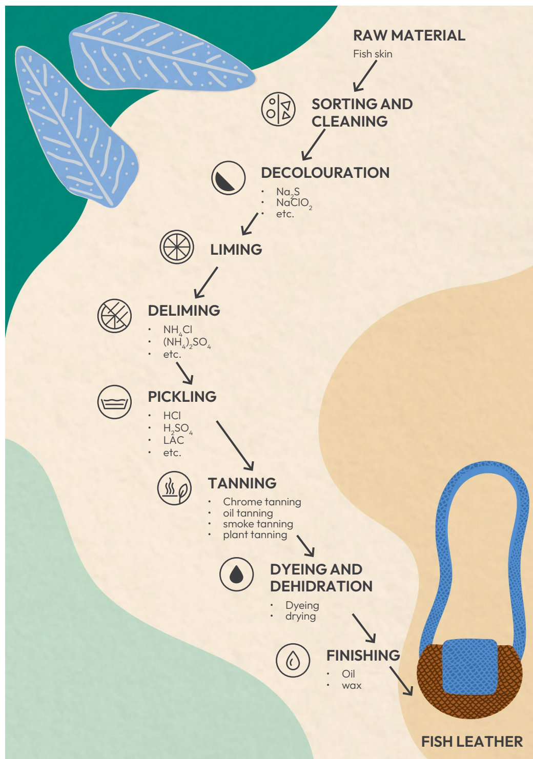
FIGURE 12. Schematic diagram of fish leather production using the by-products of aquatic food processing
