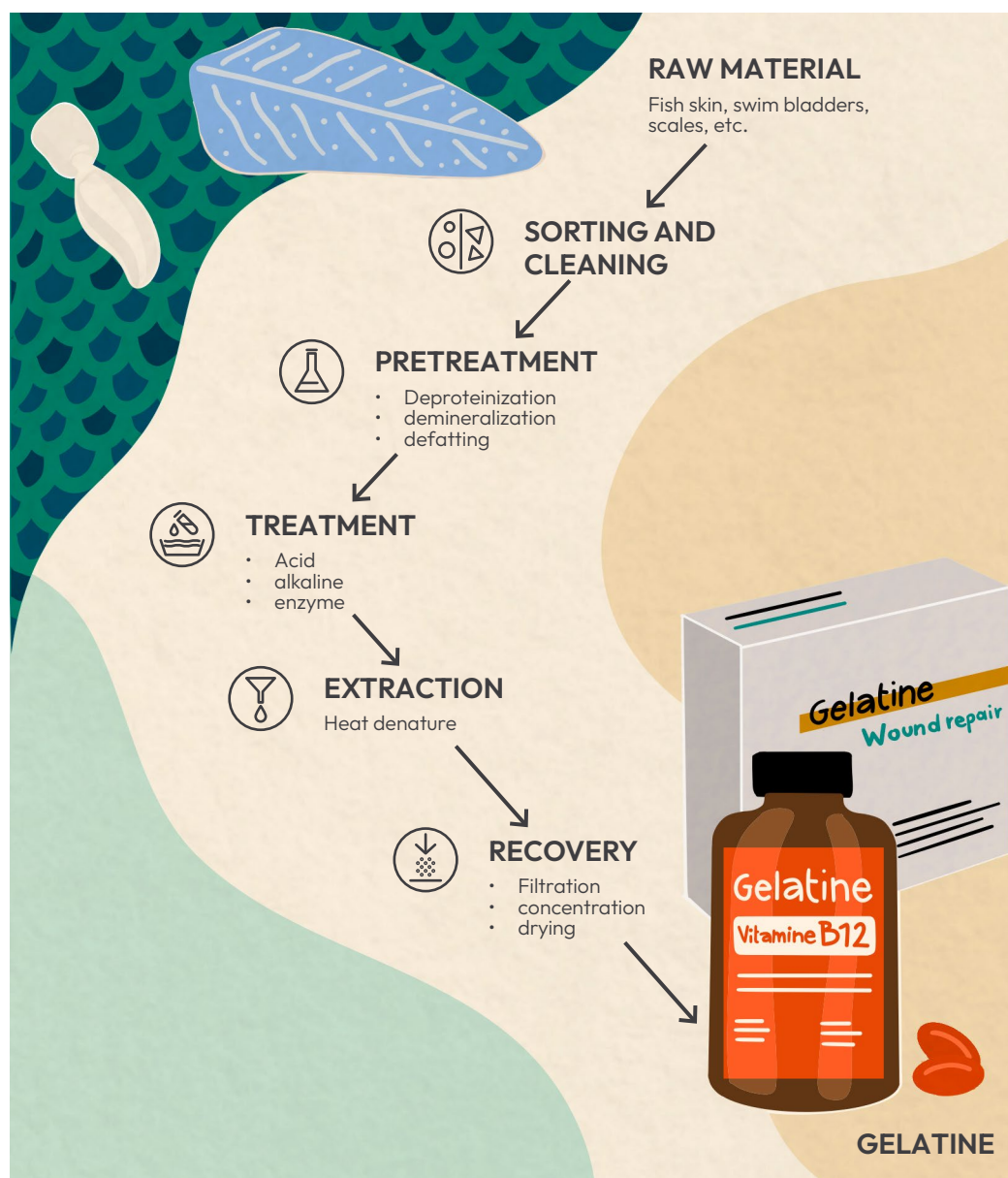
FIGURE 4. Schematic diagram of gelatine production using by-products of aquatic food processing
