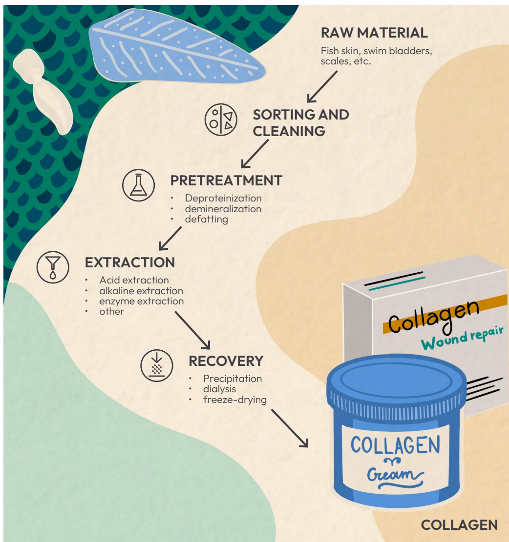
FIGURE 3. Schematic diagram of collagen production using the by-products of aquatic food processing
